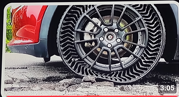
Michelin Airless Tire UPTIS - Unique Puncture-Proof Tire
