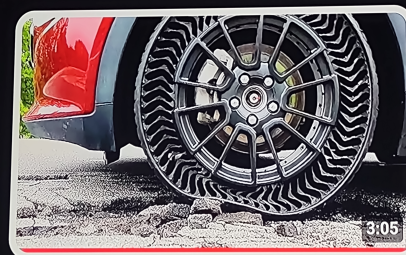
Michelin Airless Tire UPTIS - Unique Puncture-Proof Tire Airless Tires
