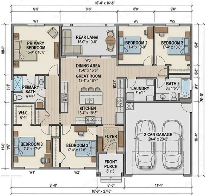
FLOOR PLAN: LEVEL 1 (1500 SQ. FT. LIVING AREA) 18'-8" x 30'-0"
