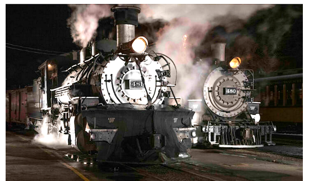
Durango & Silverton Narrow Gauge Railroad K36-class 2-8-2 engines No. 481 and 480 (both Baldwin Locomotive Works, 1925) pose at the Durango, Colo., depot the night before No. 481 led a photo special. Dan Cupper, Train.com
