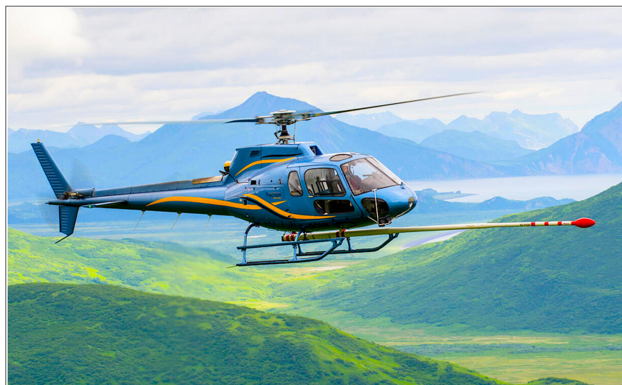
Photo: This AS350 helicopter is fitted out for an airborne geophysical survey with instruments in a long "stinger" that juts out in front of the helicopter to get the equipment as far from the rotor blades and the electrical instruments in the cockpit of the helicopter. Image courtesy of Erik Keyser of Precision GeoSurveys.
